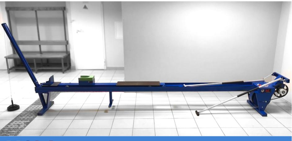
When working on this training machine, paddlers must do the following: a canoeist must get down on his knees on a special platform attached to a cart with 4 wheels and move forward and backward along the frame, performing the same movements as in a canoe in smooth water.
