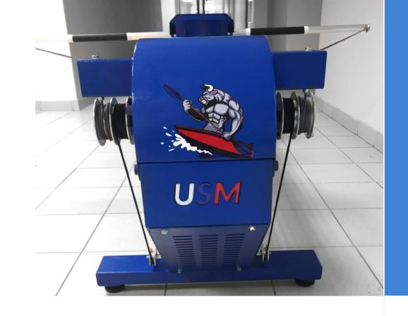
It is intended for the advancing the kayaking technique, as well as for the developing a special physical training of kayakers and testing them for a special physical condition. When working on this training machine, a kayaker must sit on a sliding seat (a seat similar to the seat located in a single kayak in smooth water) attached to a cart with 10 wheels, and move forward and backward along the frame.
