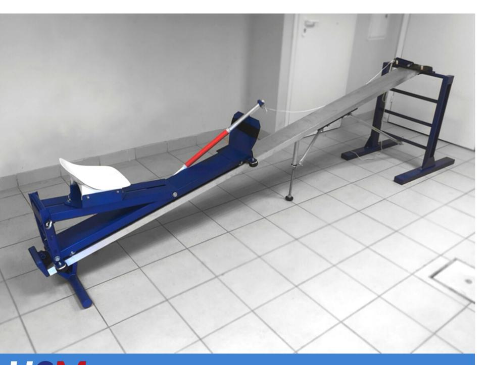
The training machine allows the paddlers to feel the transfer of force from the paddle to the kayak.
